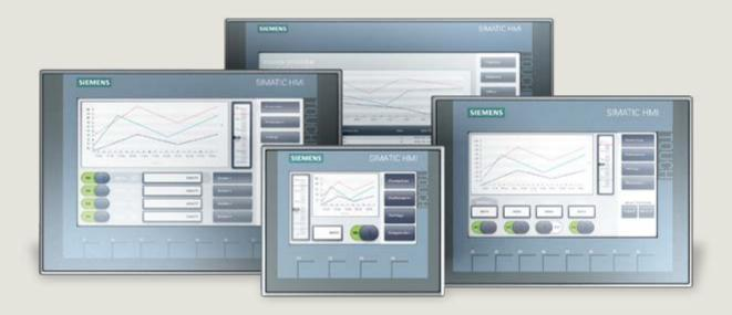
Basic Panels are made for the cost-effective implementation of simple visualization tasks on the machine level. Their basic features and functionality as well as the especially attractive price make them perfect entry-level devices.
